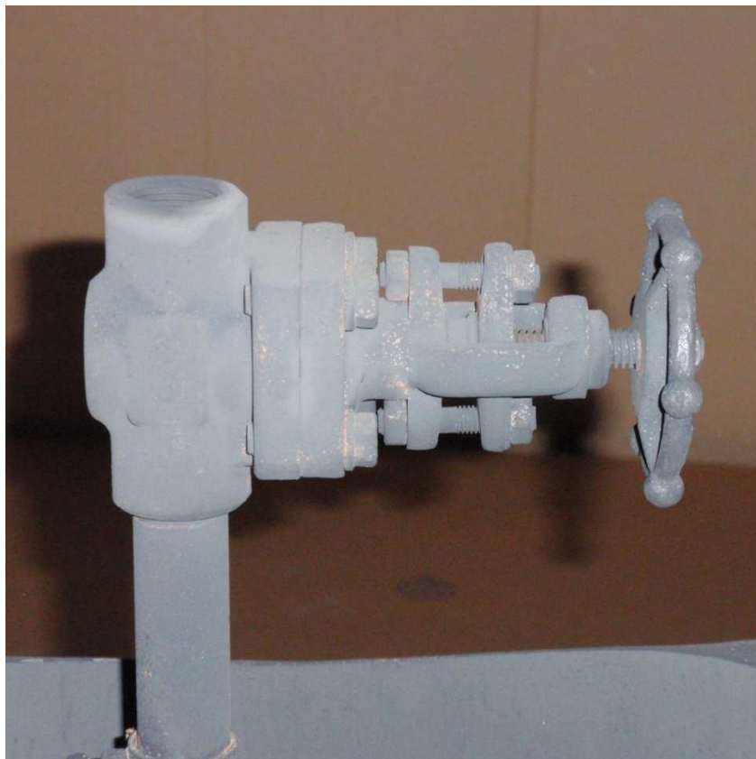
Figure 11: Prop Propane Service Valve
