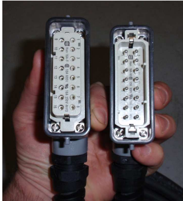
Figure 7: Detail of Control Cable ends
